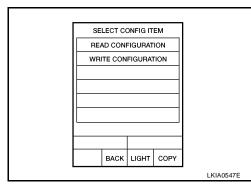
Configuration of current BCM is printed out automatically. A listing of manual setting items and auto setting items will be displayed. Auto setting items are preset and cannot be changed. Manual setting items can be set by using WRITE CONFIGURA-TION PROCEDURE. Refer to BCS-23, "WRITE CONFIGURA-TION PROCEDURE".
