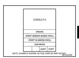
3. Touch "BCM" on "SELECT SYSTEM" screen. If "BCM" is not indicated, go to GI section. Refer to GI-40, "CONSULT-II Data Link Connector (DLC) Circuit".
