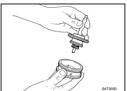
6. Install D-ring (1) to OD servo piston (2).
