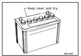
When the vehicle is not going to be used over a long period of time, disconnect the negative battery terminal.
