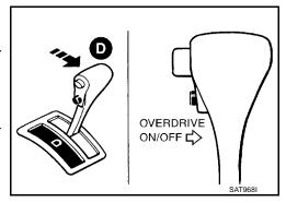
11. Depress and hold the overdrive control switch (the O/D OFF indicator lamp will be OFF) until directed to release the switch.
