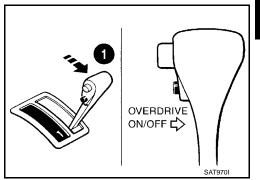
Release the overdrive control switch (the O/D OFF indicator lamp will begin to flash ON and OFF).
