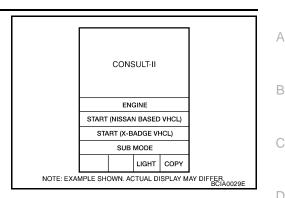
3. Touch "BCM" on "SELECT ITEM" screen. If "BCM" is not indicated, go to GI section to check CONSULT II data link connector (DLC) circuit. Refer to GI-41, "CONSULT-II Data Link Connector (DLC) Circuit".
