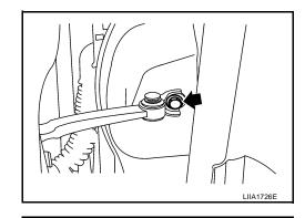
Remove the door hinge nuts, and remove the door assembly.
