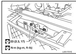
Removal and Installation of Hood Assembly
