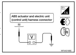
Check resistance between ABS actuator and electric unit (control unit) harness connector E125 and body ground.
