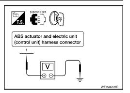
Check resistance between ABS actuator and electric unit (control unit) connector E125 and body ground.
