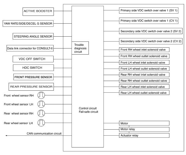
ABS actuator and electric unit (control unit)
