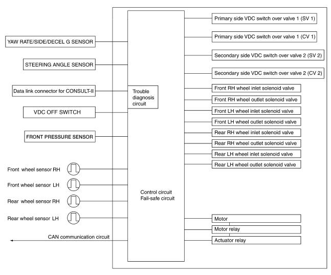
ABS actuator and electric unit (control unit)
