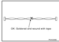
Do not make a bypass connection to repaired area. (If the circuit is bypassed, characteristics of twisted wire will be lost.)
