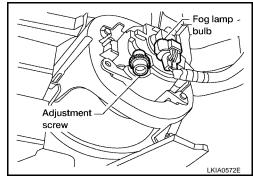
• Use adjustment screw so that the top edge of the high intensity zone is 100 mm (4 in) below the height of the fog lamp centers as shown.
