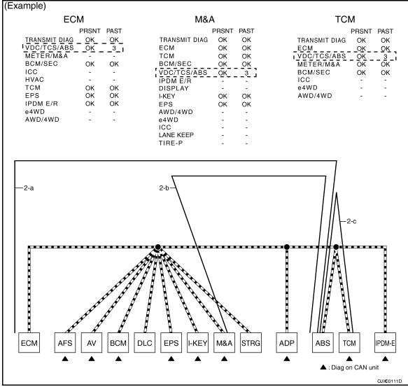
CAN DIAG SUPPORT MNTR (without PAST): Check the CAN DIAG SUPPORT MNTR (without PAST) of units indicating "U1000" or "U1001" on SELF-DIAG RESULTS. Draw a line on the diagnosis sheet to indicate the possible error circuit.
