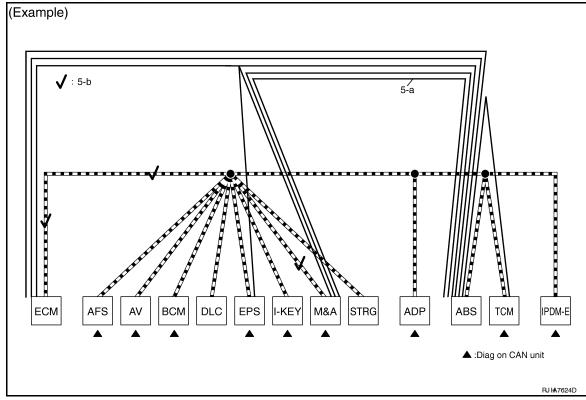
The circuit which has the most amount of lines are the possible cause. Error is detected from ABS actuator and electric unit (control unit) branch line (shaded in the figure below).
