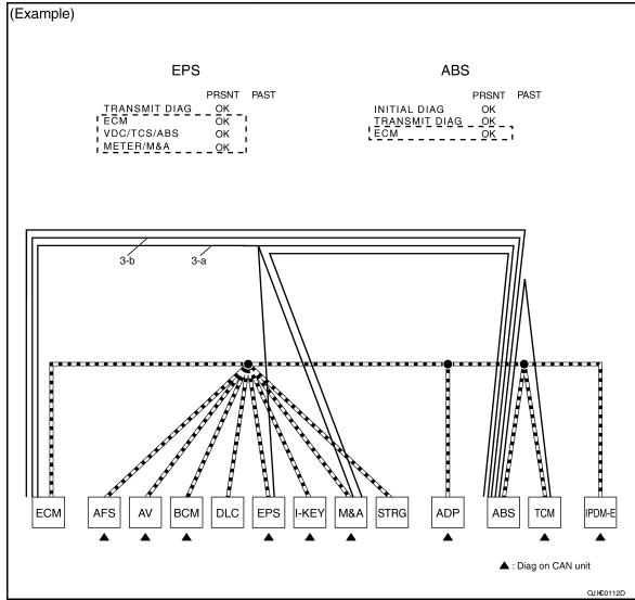
Search for the possible cause using CAN communication signal chart using information from the interview with the customer.
