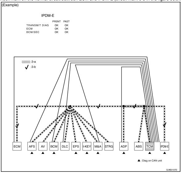
4. Through the above procedure, the error is detected in the TCM branch line (shaded in the figure below).
