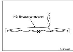
• Replace the applicable harness as an assembly if error is detected on the shield lines of CAN communication line.
