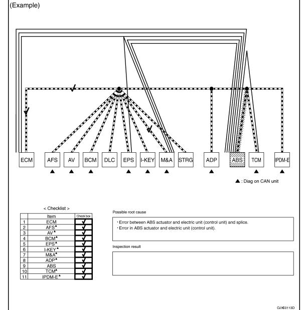
Past Error — Short Circuit — When the symptoms listed below exist, a short circuit of the CAN communication line is a possible cause.
