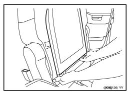
3. Hold the seatback board as shown and pull the bottom of the seatback board away from the seat back frame.
