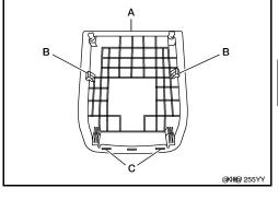
Hold the seatback board as shown and pull the top of the seatback board away from the seat back frame.
