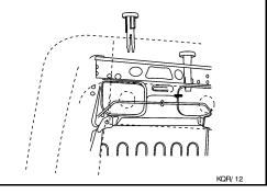
Remove the snap ring and the lumbar support lever knob (if equipped).
