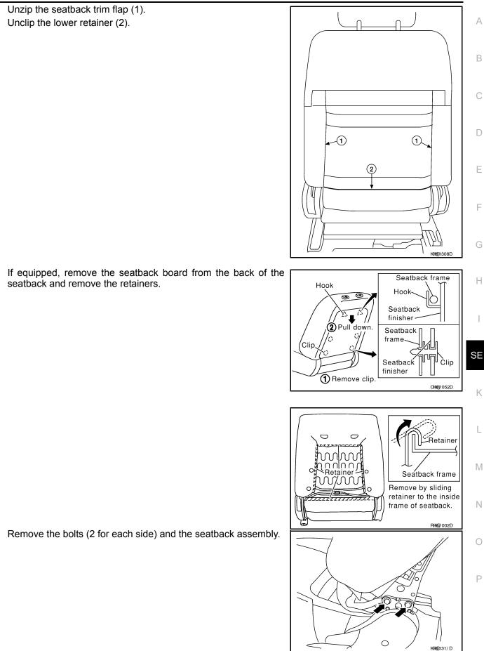
5. Remove the bolts (2 for each side) and the seatback assembly.
