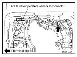
6. Remove A/T fluid temperature sensor 2 with bracket from control valve with TCM.
