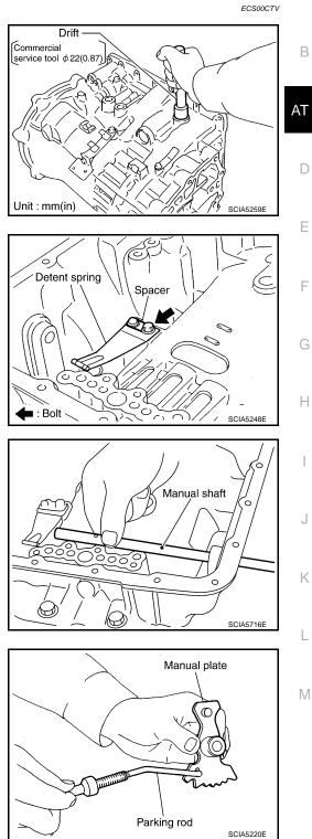
5. Install manual plate (with parking rod) to manual shaft.
