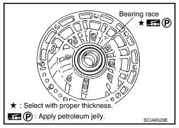
2. Install bearing race to oil pump assembly.
