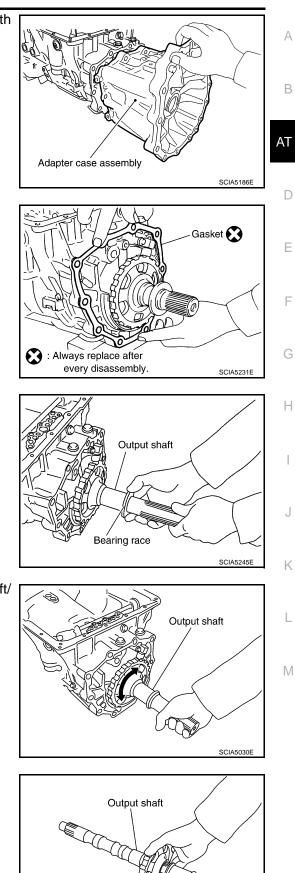
47. Remove seal rings from output shaft.
