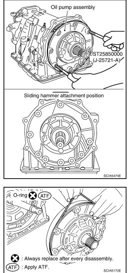
9. Remove bearing race from oil pump assembly.
