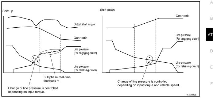
\*1: Full phase real-time feedback control monitors movement of gear ratio at gear change, and controls oil pressure at real-time to achieve the best gear ratio.
