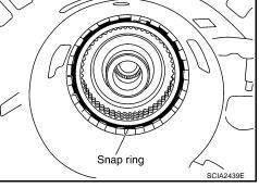
21. Install snap ring in transmission case.
