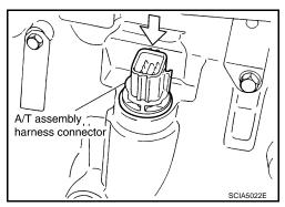
5. Push A/T assembly harness connector. **CAUTION:** Be careful not to damage connector.
