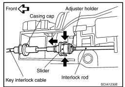
3. Remove holder from key cylinder and remove key interlock cable.
