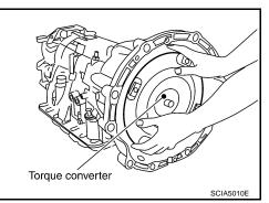
c. Measure distance "A" to make sure that torque converter is in proper position.
