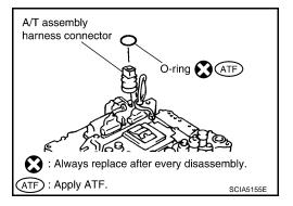
5. Install A/T fluid temperature sensor 2 to bracket.
