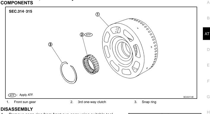
1. Remove snap ring from front sun gear using suitable tool.
