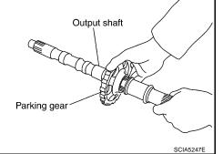
31. Install output shaft in transmission case.
