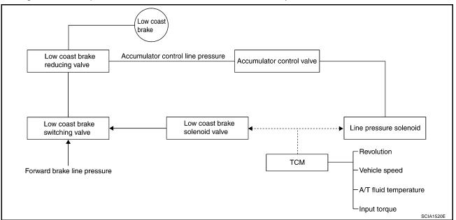
The operation of the low coast brake solenoid switches the low coast brake switching valve and controls the coupling and releasing of the low coast brake.
