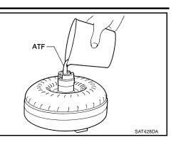
b. Install torque converter while aligning notches of torque converter with notches of oil pump.
