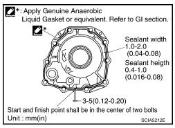
ii. Install rear extension assembly to transmission case.
