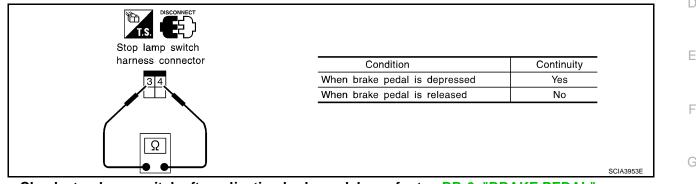
Check stop lamp switch after adjusting brake pedal — refer to BR-6, "BRAKE PEDAL".
