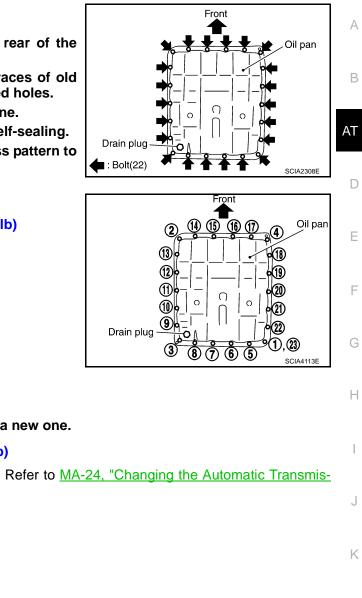
4. Install drain plug to oil pan.
