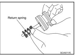
9. Install return spring to servo assembly.
