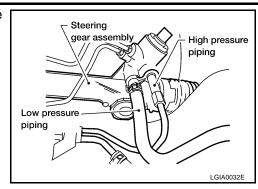
10. Remove the bolt from the lower joint of the lower joint shaft, then separate the lower joint from the steering gear assembly.
