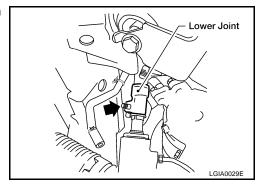
11. Remove the nuts and bolts of the steering gear assembly, using power tool, then remove the steering gear assembly from the vehicle.
