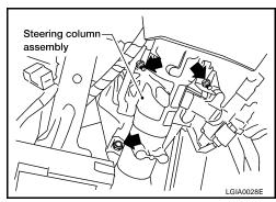
9. Remove the bolt from the lower joint of the lower joint shaft, then remove the lower joint shaft from the vehicle.
