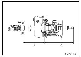
3. Check the tilt device for proper operation range.
