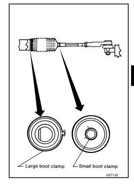
5. Crimp the large-diameter boot clamps, using Tool.
