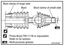
4. Install the boot clamps to the boots, as shown.
