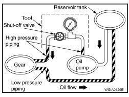
Start the engine. Run the engine until the power steering fluid temperature reaches 50 – 80°C (122 – 176°F).
